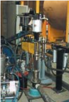
Piston and diaphragm pumps used for two-component paint machines.
