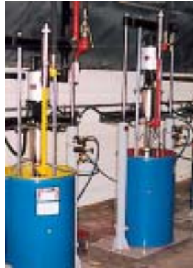
Extrusion pumps & accessories used for thick sheet fed inks.
